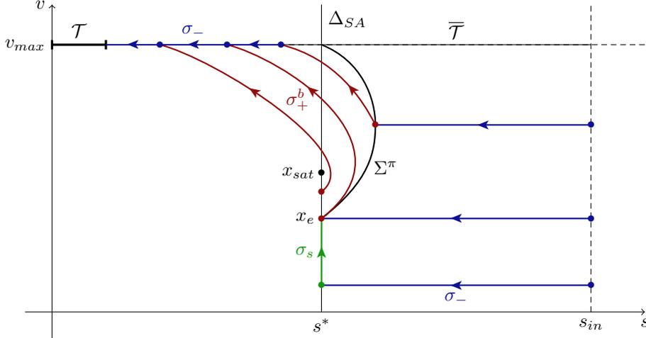
Figure 3: Minimal time synthesis for (5.2): the target set  $\mathcal{T} = (0, s_{ref}] \times \{v_{max}\}$  is in black (left). The switching curve  $\Sigma^\pi$  (in black) is tangent to the bridge  $\sigma_+^b$  (in red) at  $x_e$ . Arcs with  $u = +1$  (resp.  $u = -1$ ) are depicted in red (resp. in blue).
